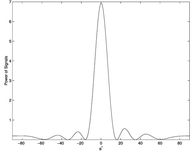
Fig. 1. Response of the spatial matched filter  $\mathbf{r}_{x_0 d_0}$ . The direction of a single incident signal is  $0^\circ$ , the number of sensors is 8, and SNR equals 0 dB.
