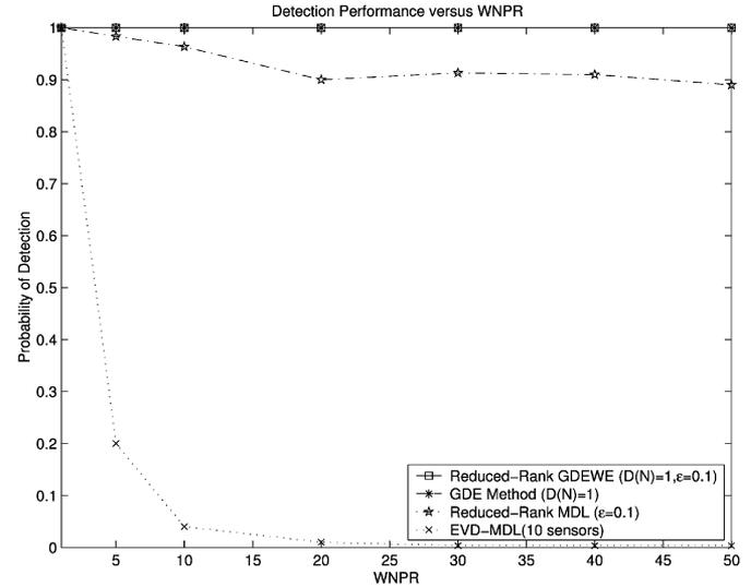
Fig. 10. Probability of correct detection versus WNPR.  $[\theta_1, \theta_2] = [0.5^\circ, 6.2^\circ]$ , SNR = 5 dB,  $N = 256$ ,  $L = 10$ , and WNPR varies from 1 to 50.
