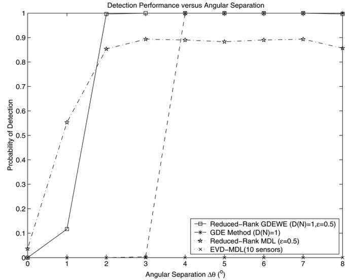
Fig. 9. Probability of correct detection versus angular separation in the case of spatially inhomogeneous noise.  $[\theta_1, \theta_2] = [0.5^\circ, \theta_1 + \Delta\theta]$ , SNR = 10 dB,  $N = 256$ , WNPR = 10,  $L = 10$ , and  $\Delta\theta$  varies from  $0^\circ$  to  $8^\circ$ .
