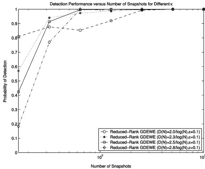
Fig. 5. Probability of correct detection of the GDEWE versus number of snapshots for different  $\kappa$  in the case of spatially white noise.  $[\theta_1, \theta_2] = [0.5^\circ, 6.2^\circ]$ , SNR = 0 dB,  $L = 10$ , and  $N$  varies from 16 to 1024.
