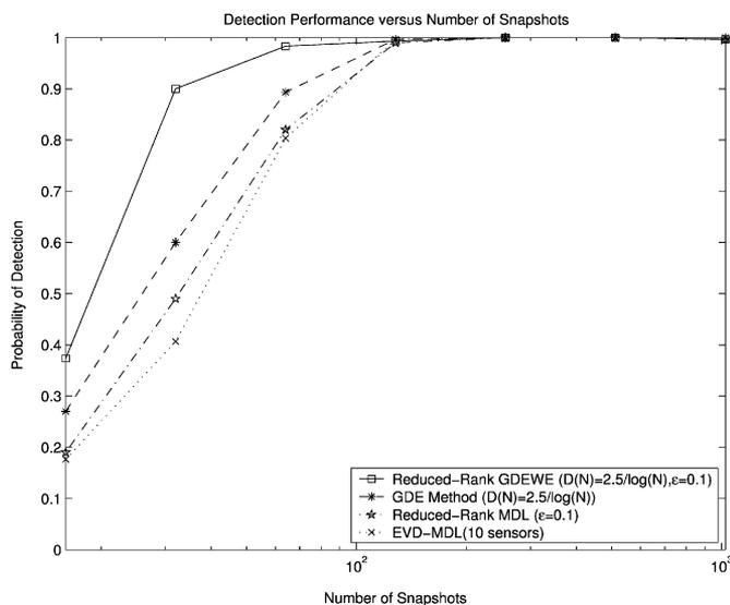
Fig. 6. Probability of correct detection versus number of snapshots for the case of spatially white noise.  $[\theta_1, \theta_2] = [0.5^\circ, 6.2^\circ]$ , SNR = 0 dB,  $L = 10$ , and  $N$  varies from 16 to 1024.
