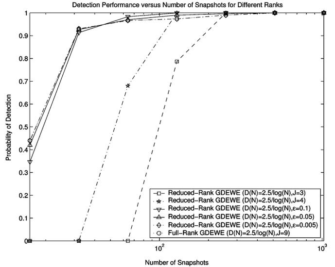
Fig. 4. Probability of correct detection of the GDEWE method versus number of snapshots for different ranks in the case of spatially white noise.  $[\theta_1, \theta_2] = [0.5^\circ, 6.2^\circ]$ , SNR = 0 dB,  $L = 10$ , and  $N$  varies from 16 to 1024.
