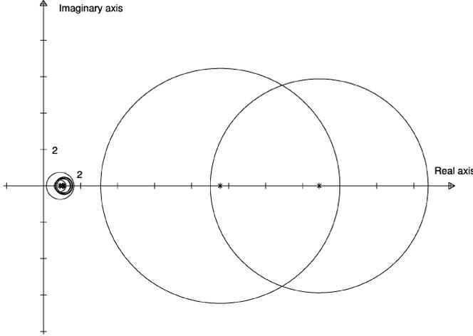
Fig. 3. Gerschgorin disks of the calculated tridiagonal matrix. \* denotes the centers of the Gerschgorin disks.
