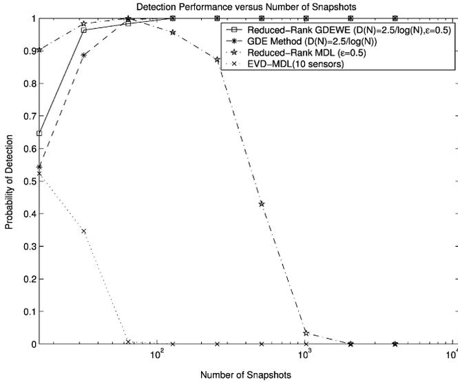
Fig. 8. Probability of correct detection versus number of snapshots in the case of spatially inhomogeneous noise.  $[\theta_1, \theta_2] = [0.5^\circ, 6.2^\circ]$ , SNR = 5 dB, WNPR = 10,  $L = 10$ , and  $N$  varies from 16 to 4096.
