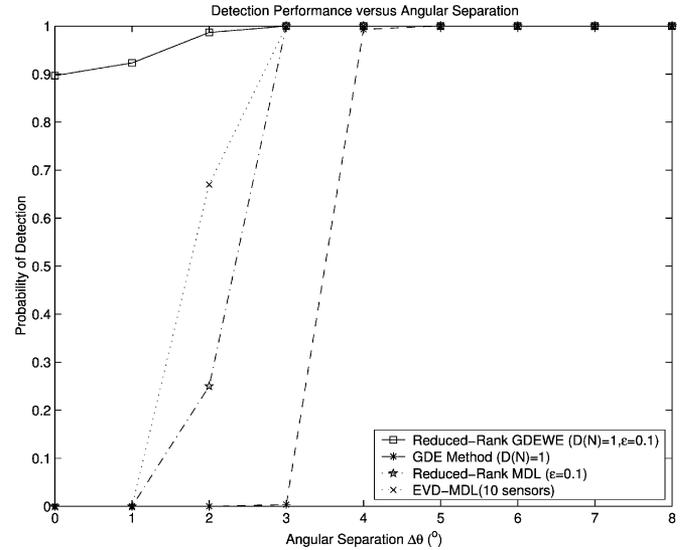
Fig. 7. Probability of correct detection versus angular separation ( $\Delta\theta$ ) for the case of spatially white noise.  $[\theta_1, \theta_2] = [0.5^\circ, \theta_1 + \Delta\theta]$ , SNR = 5 dB,  $N = 256$ ,  $L = 10$ , and the angular separation varies from  $0^\circ$  to  $0^\circ$ .
