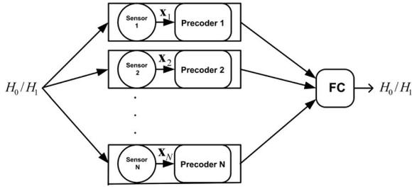
Fig. 1. Decentralized detection of unknown deterministic vector signal. Each node processes its vector observations through linear precoder. Messages are then sent to FC to form final decision.
